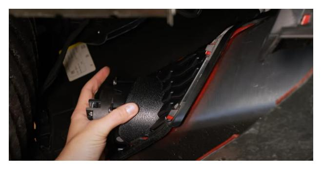
Back at the vehicle, place the assembled bezels into the original equipment (OE) position on the bumper.
