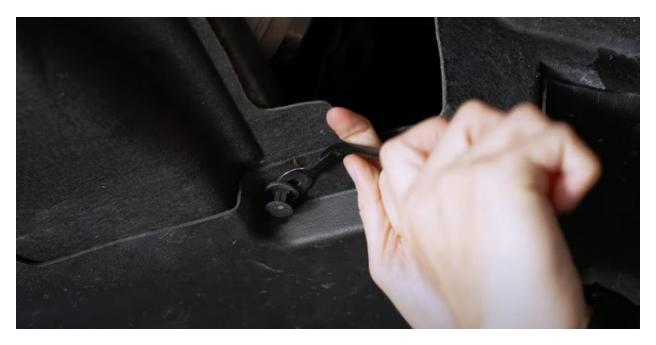
Next, use a **trim removal tool** to remove the **three push pins** holding the shield.
