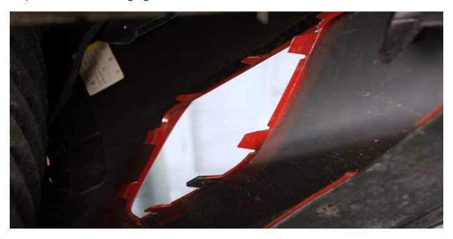
With the grilles removed, it's time to assemble the fog lights and bezels.
