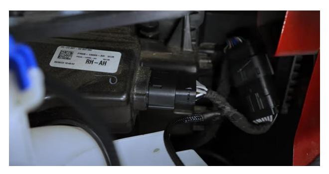
Behind the **passenger-side headlight**, disconnect the OE harness and connect the fog light harness in line.
