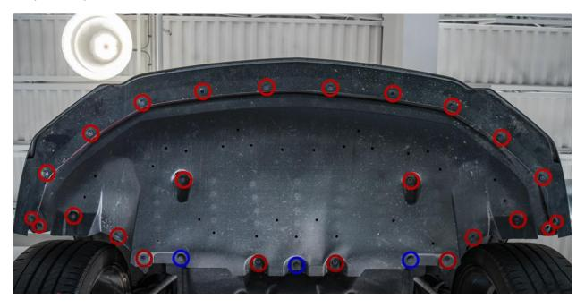
Begin by removing the necessary components from underneath the vehicle to access the fog light installation area. Using a **7mm socket**, remove **24 screws** securing the shield in place.
