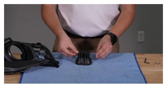
**-If using SS3 pods**: Assemble the pods by placing the supplied **locking nuts** into the back of the pod with the nylon ring facing inward.
