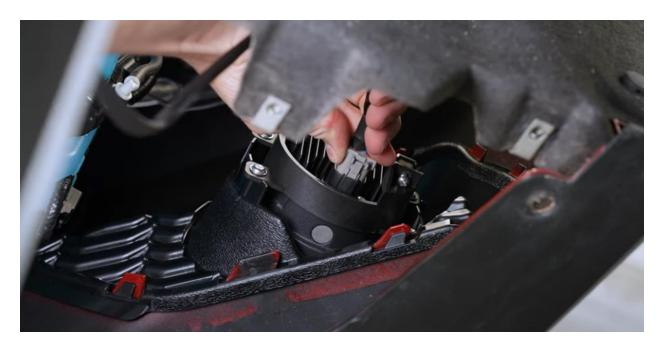
Attach the **shorter DT output lead** to the passenger-side fog lamp. Route the **longer DT lead** across the radiator subframe and connect it to the driver-side fog lamp.
