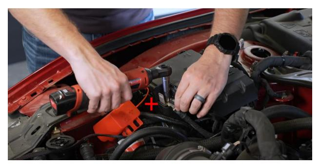
In the engine bay, locate the fuse bus in front of the fuse box. Use a **10mm socket** to loosen the positive connection and attach the **positive lead** from the fog light harness.
