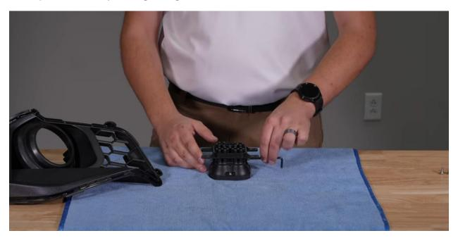
Slide the **Type A mounting bracket** over the pod and secure it using a **5/32-inch Allen screw** and washer.
