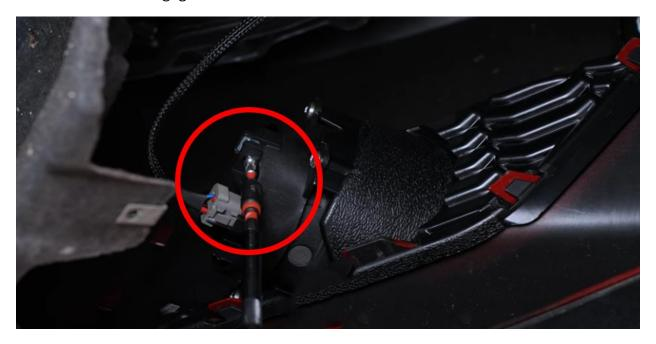
If adjustments are needed, use a **Phillips head screwdriver** to turn the adjustment screw and aim the fog lights properly.
