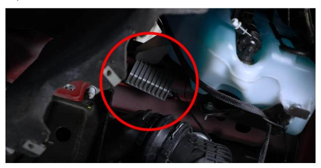
With everything functioning correctly, secure the solid-state relay and any loose wiring using zip ties. Ensure all components are routed away from hot or moving parts. Finally,
