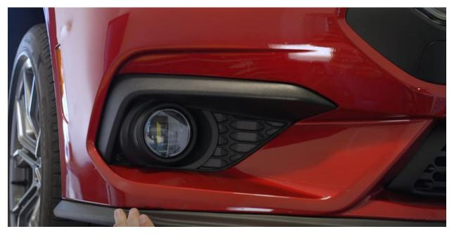
Press firmly to ensure all retaining clips are seated properly. Repeat this step for the second bezel.
