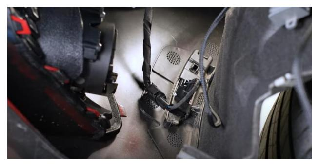
Then connect the fog light harness in line with the OE harness.
