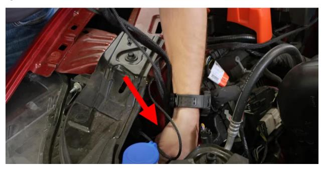
Route the remaining harness behind the headlight, ensuring it is kept away from hot or moving parts.
