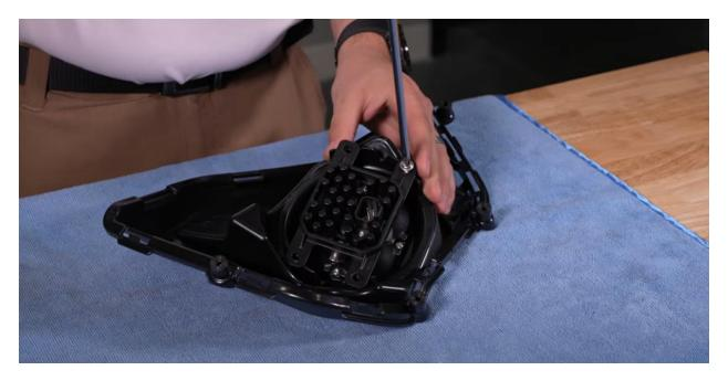
Then, secure the pod to the bezel using the **four included screws** and a **Phillips head screwdriver**.
