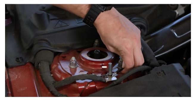
Then, use an **8mm socket** to attach the **negative lead** to the ground stud located on top of the strut tower.
