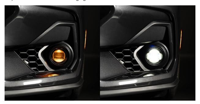
Once the harness is fully connected, test the functionality of the fog lights. The **amber backlight** should activate with the parking lights, and the **main beam** should turn on when the low beams are engaged.
