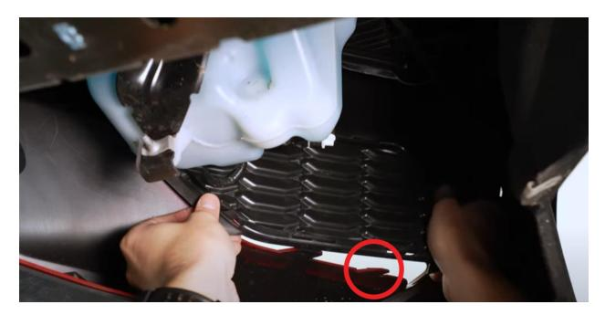
Behind the grille, use your hands to release the **10 retaining clips** that secure the side corner grille in place. Apply outward pressure to each clip while simultaneously pulling the grille toward the rear of the vehicle. Repeat this process for both sides of the vehicle.
