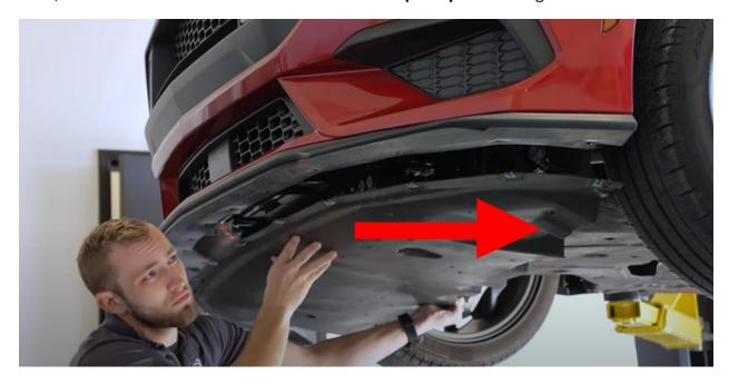
Once these fasteners are removed, slide the shield toward the rear of the vehicle to release it.
